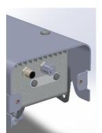
This will reveal an aluminium panel secured with two Torx screws—this is the SIM card cover.
