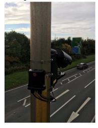
The Rapier 250/350IQ is built upon the already successful camera and illuminator combination from the Rapier 50, which is capable of reading number plates up to 50m (250IQ) or 30m (350IQ) and provide night-time visible make and model monochrome images from the overview camera at distances up to 25m. Both cameras are fitted with motorised zoom lenses, providing 8m (250IQ) and 12m (350IQ) field of view.
