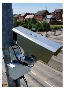
The unit also supports a remote power reset to reboot the system and a hardware watchdog timer to automatically reboot the system in the event it has become unresponsive, ensuring operational capabilities are not compromised for any length of time.
